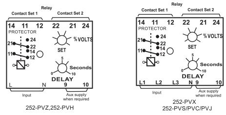
Note : The neutral connection is always used on 4 wire system
